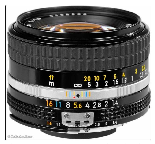
The f stops are colour coded to save space only. In the picture the lens is focused at infinity and f5.6 has been selected. (The black dot is the focus point for ordinary film, the red dot for infrared film.)
